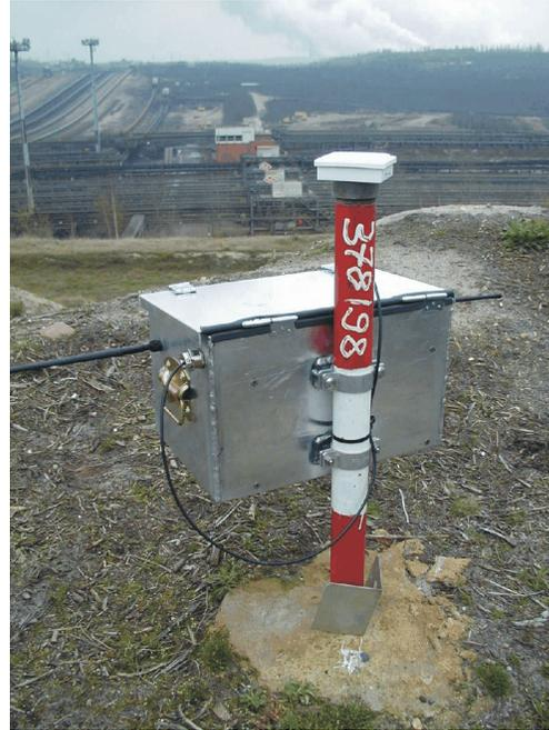
**Fig. 2** Example of a GPS receiver and telemetric equipment within a GOCA sensor array in case a slope monitoring in open cast mining at RWE Power AG (see, tab. 1) using the GOCA system.
