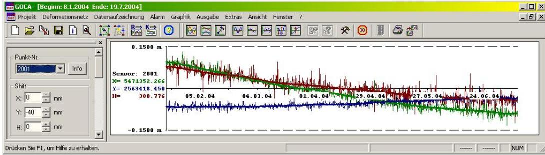
**Fig. 3** GOCA object-point time series  $\mathbf{x}_o(t_i)$  as result of the 2<sup>nd</sup> adjustment step of the GOCA-software. The thick lines show the smoothing by a robust moving average estimation applying the M-estimation (5c).
