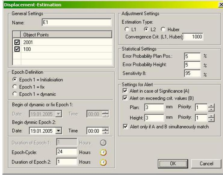
Fig. 4. GOCA online deformation (3<sup>rd</sup> step). Settings for the online displacement estimation and alerting.
