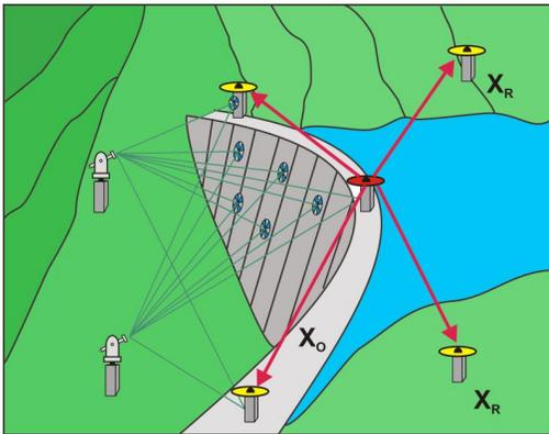
**Fig. 1** Design of a classical absolute deformation network realized by the GOCA system.
