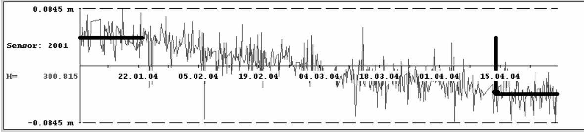
**Fig.5** Visualization of the GOCA displacement estimation (3<sup>rd</sup> step). Thick horizontal line left shows the estimation of  $\mathbf{x}_0$  (8a), (8b) by a number of observations  $\mathbf{x}_0(t_i)$  belonging to the reference time  $t_0$ . The thick horizontal line right shows the estimated position  $\mathbf{x}(t) = \mathbf{x}_0 + \mathbf{u}(t)$ , and the thick arrow shows the estimation vertical displacement  $\mathbf{u}(t)$ .
