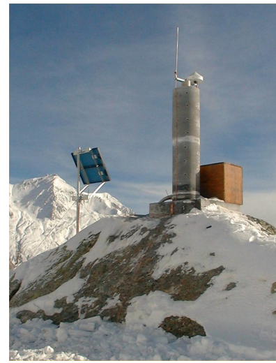
Fig. 7: GPS-receiver on pillar with solar panel energy supply as part of the GOCA array for the monitoring of the Gotthard railway tunnel construction (2002-2014).
